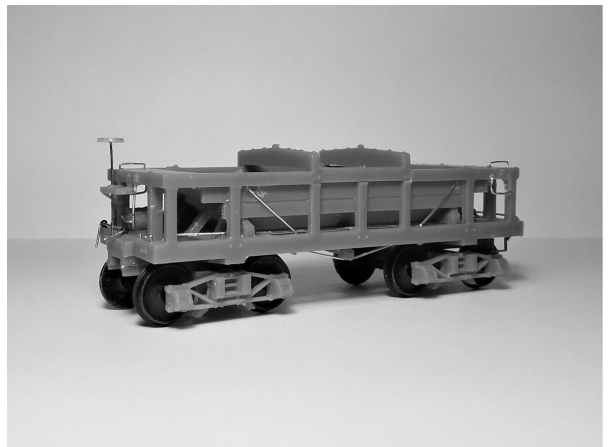
Completed DM&N Class R body showing Truss Rod and Train Line position.
