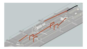
17. **Brake beam hangers:** these cars had body-hung brake beams. Replicating the hangers is difficult and may cause issues during operation. If you wish to add them, see the diagram below. We supplied eye bolts for this. Bend pieces of wire about 2 feet in length with the tips curved to connect the hangers with the brake shoes. The holes in the brake shoes may need to be drilled out. If so, be very careful and use a #79 drill bit.
