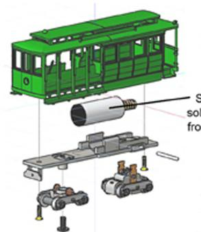
Attach trucks, then insert frame into body and attach with two 00-90 screws (not included) Note: Assembled cable car will have Shorty trucks and motor reversed, so test and verify wiring polarity.
