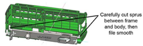
Tap body mounting screw holes for 00-90 screws Clean parts in isopropyl alcohol, dry, and paint. Add glazing
